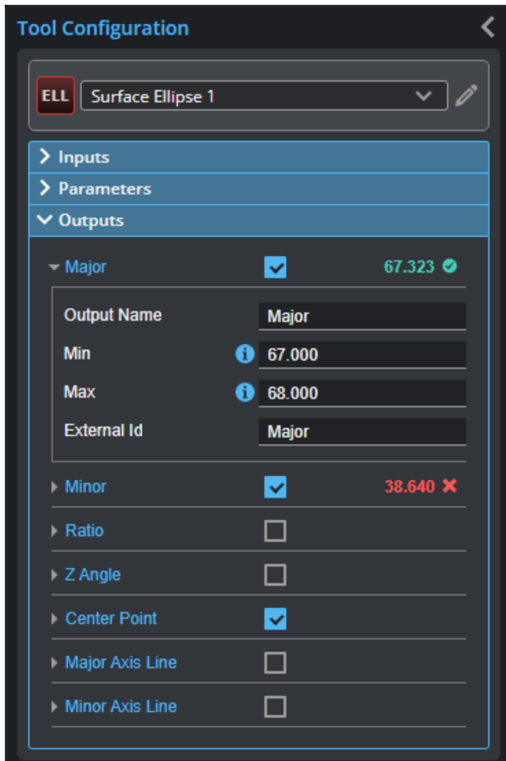
Outputs section with a measurement expanded to show user-configurable decision min/max fields and an external ID
