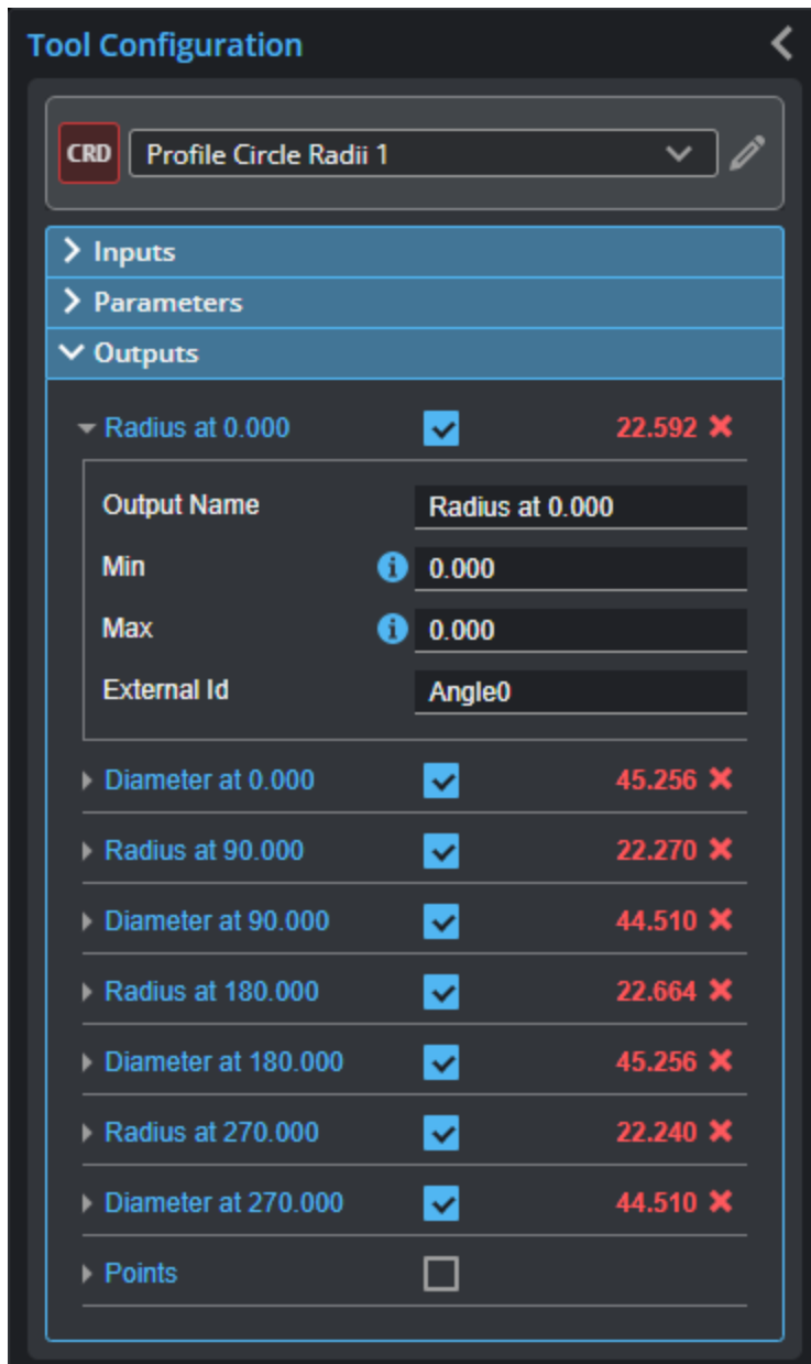
Outputs section with a measurement expanded to show user-configurable decision min/max fields and an external ID
