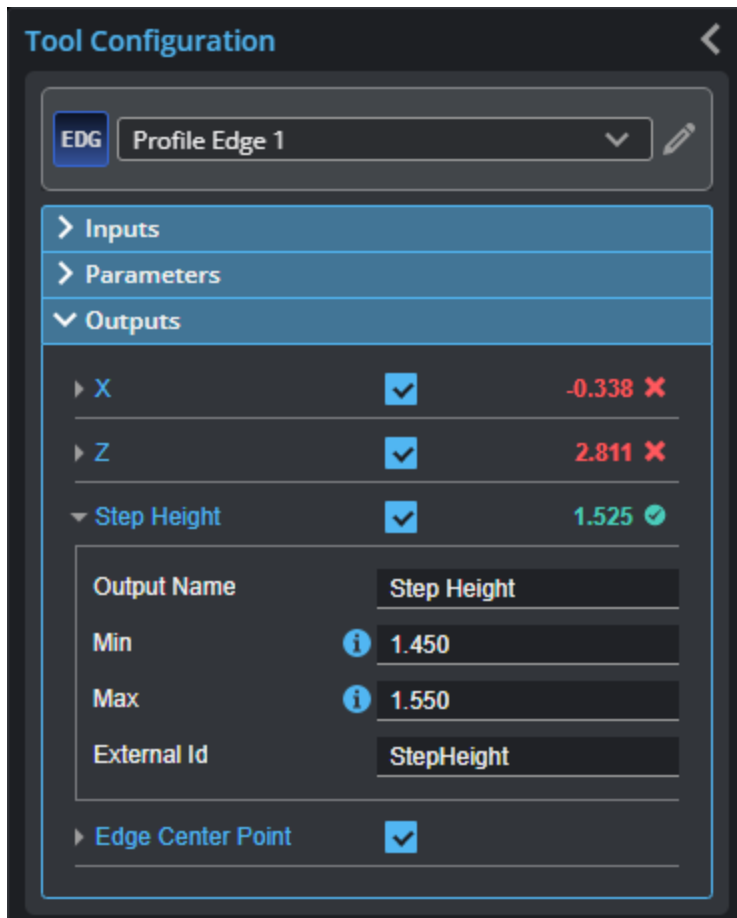
Outputs section with a measurement expanded to show user-configurable decision min/max fields and an external ID
